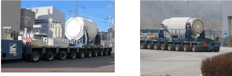
Figure 2. On-site transport between unit and the interim storage facility in Doel (left – Dual Purpose Cask for Transport & Storage) and Tihange (right – Shuttle cask)
