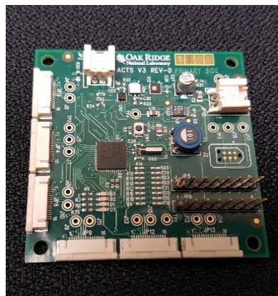
Figure 4. The low-power ACTS circuitry with sensor suite and peripheral expansion slots extends capabilities, while the inertial measurement unit senses motion to reduce power consumption and allow smarter control of the communication device's power.
