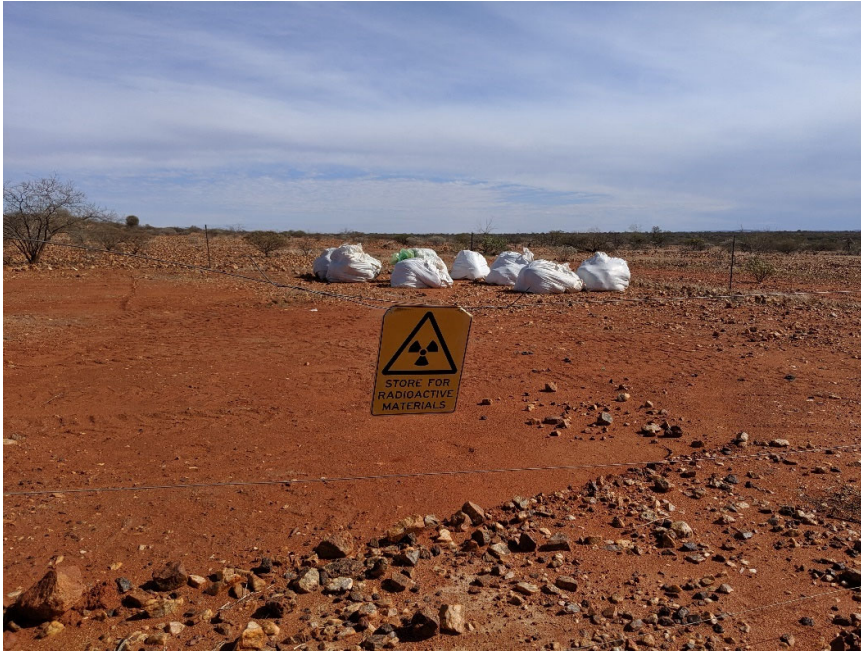
Figure 1 Radioactive store for rock samples in an area with ore body outcroppings of 4 \mu\text{Sv}/\text{Hr}
