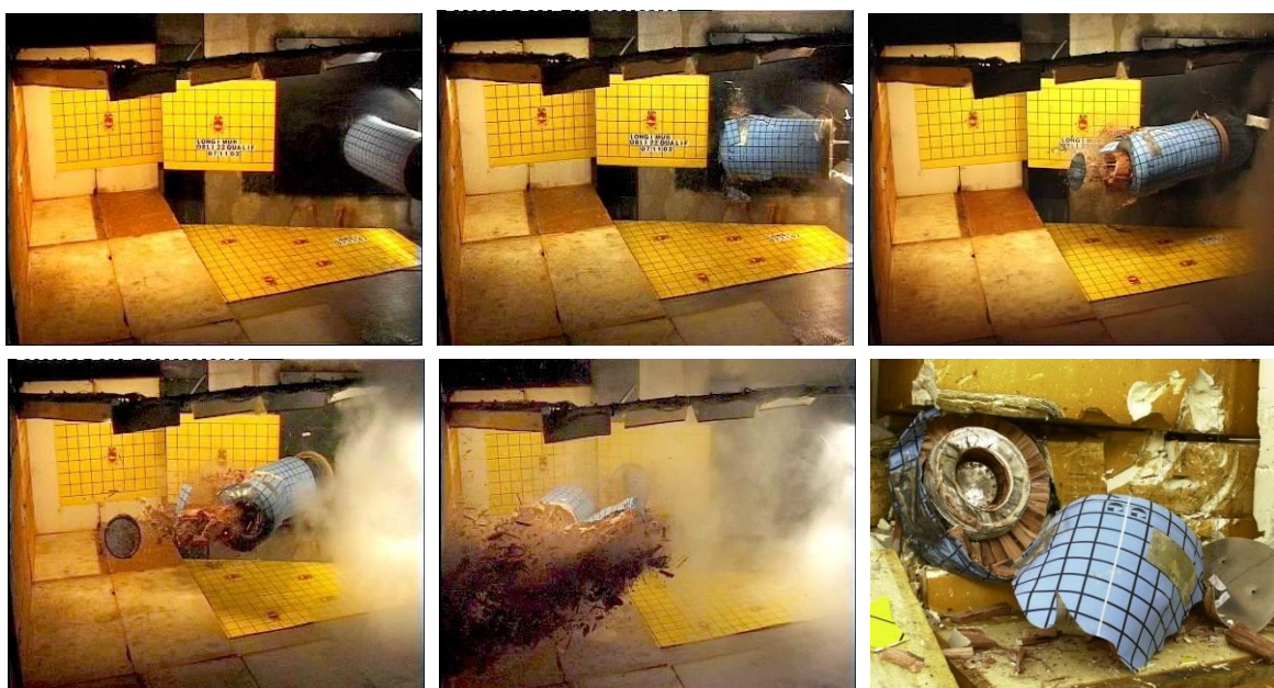
Figure 15. Impact test ( 105 \text{ m.s}^{-1} ) on a oriented target
