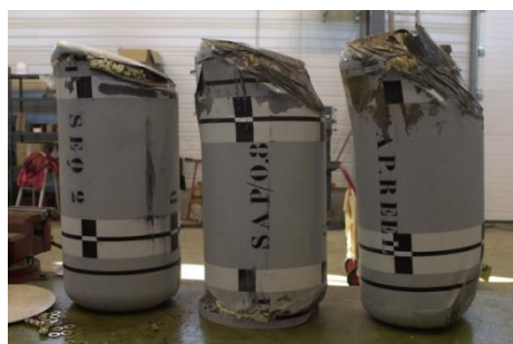
Figure 7. Three mock-up containing different type of wood (sequoia, deal, poplar) after a launch with an angle of 45^\circ
