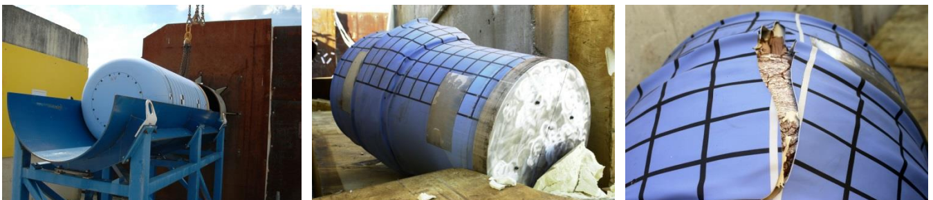
Figure 10. Package before (left) and after (center and right) the impact test in axial orientation
