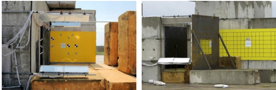
Figure 5. Views of the unyielding target (steel plate in black), sighting marks and debris stopper (right)
