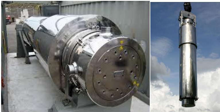
Figure 3. Vertical and Horizontal Pictures of the NAC-LWT Cask
