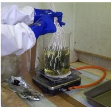
Figure 12. Removal of corrosion products
