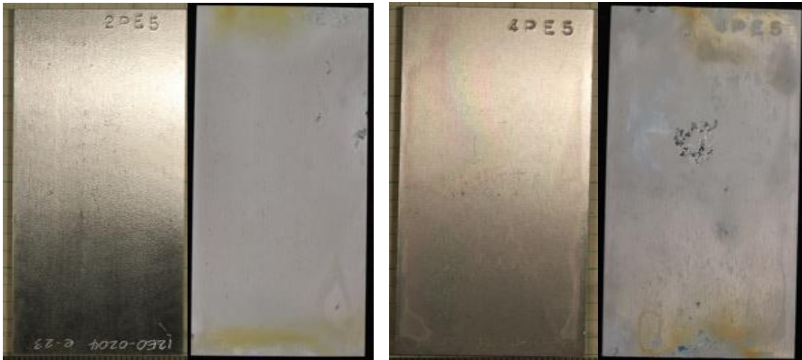
Figure 6 MAXUS® 5-Year PWR Bath Encapsulated Coupons
