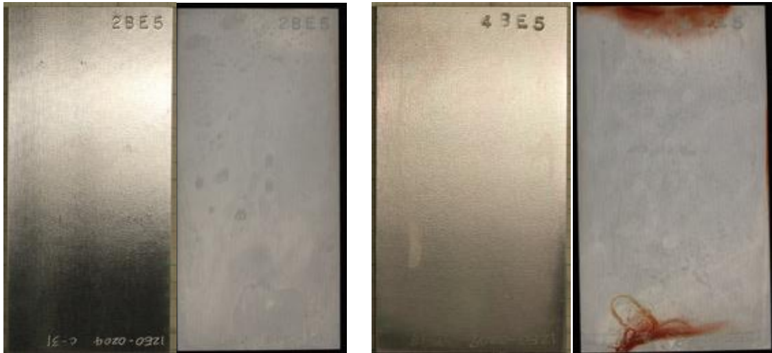
21wt% B 4 C BWR Encapsulated
