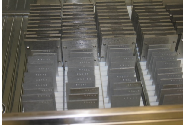
Figure 2. Bare (front) and SS encapsulated (back) BORAL ® coupons in a test bath.
