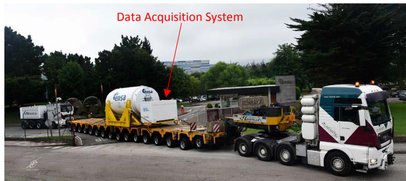
Figure 5. ENUN 32P cask on the trailer used in heavy-haul transport.
