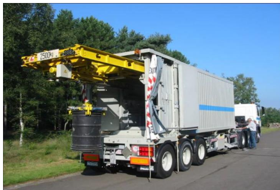
Figure 1. Shielded ISO 20ft container equipped with autonomous loading/unloading system
