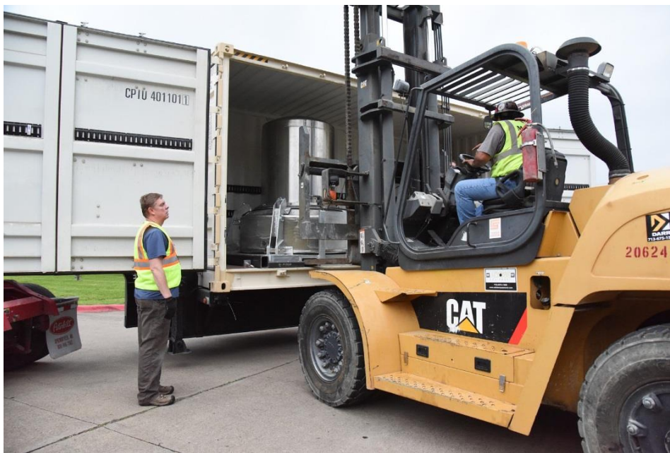
Figure 1 Using a forklift to unload a 435-B from an intermodal container
