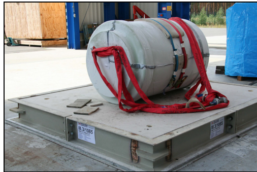
Figure 3. Cylindrical DCI cask after drop test from 0.96 m height onto a concrete target
