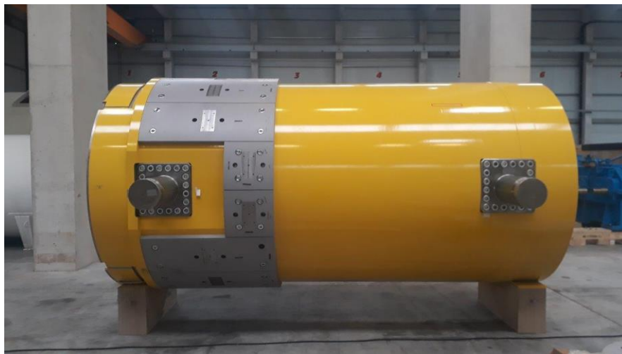
Figure 2. TGC27 Mock-up (without shock absorbers)
