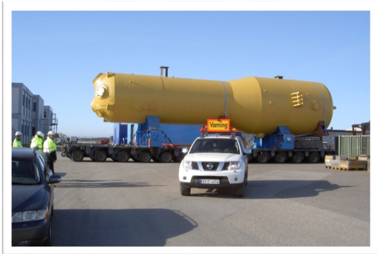
Example of radioactive waste, a discarded PWR steam generator under transport to conditioning facility (large items). Use “A” documents.
