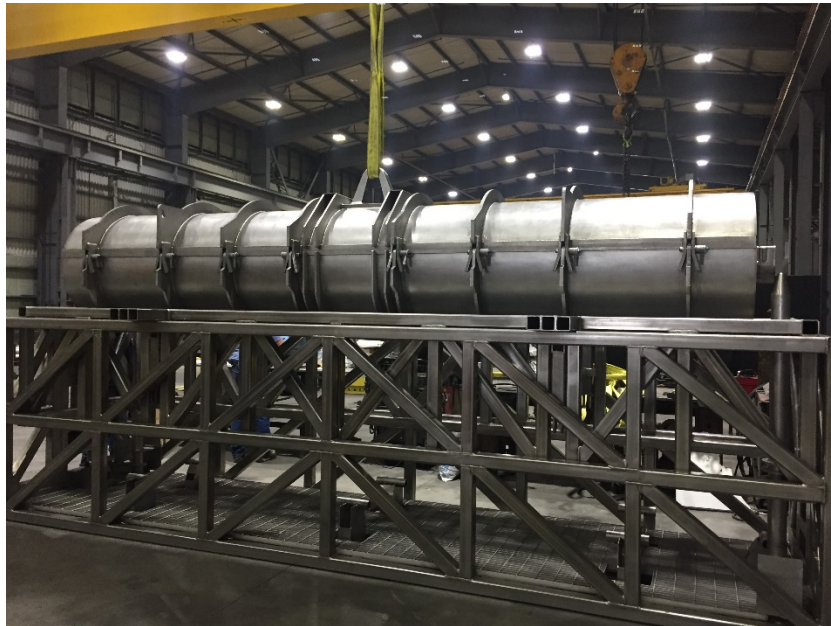
Figure 3: Mk-18A Target Shield Assembly Removed from the Cask Frame
