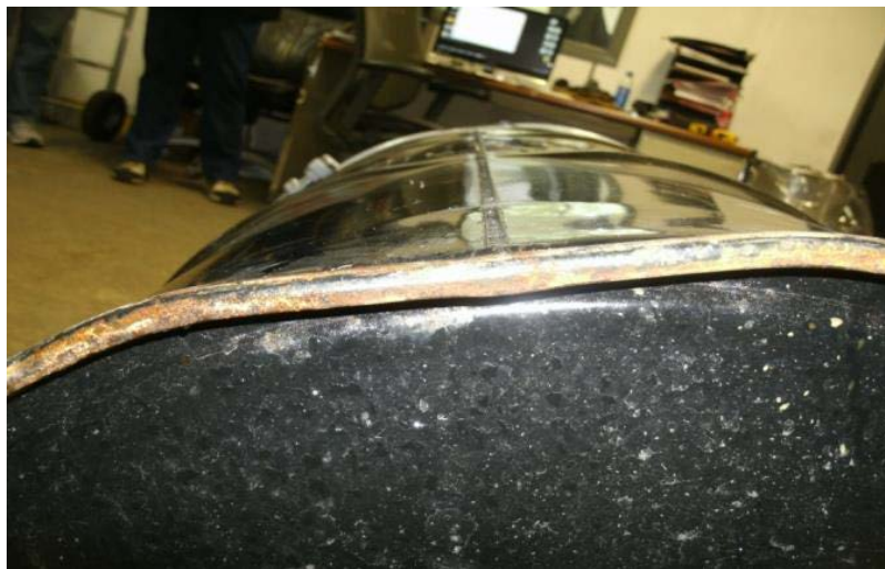
TU-1 Post Drop Damage
