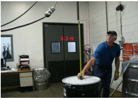
TU-2 Penetration Test
