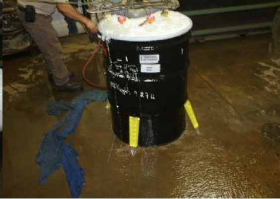
TU-1 Post Water Spray Test
