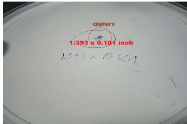
TU-2 Post Penetration Test Damage
