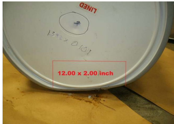
TU-2 Post Drop Test Damage
