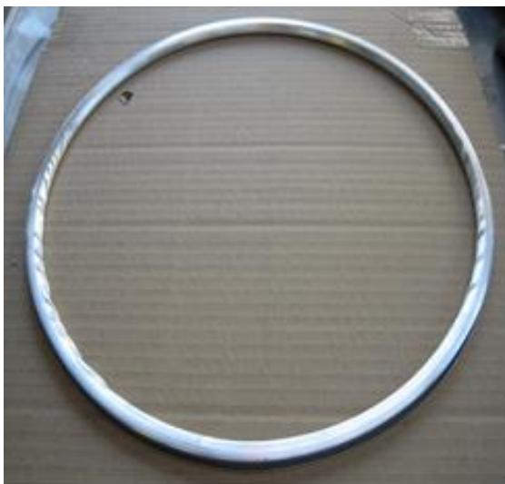
Fig. 4: HELICOFLEX type seal with typical deformation after an excessive dynamic lateral sliding
