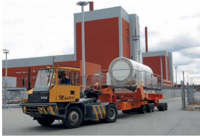
Figure 9: CASTOR ® TVO during onsite transport
