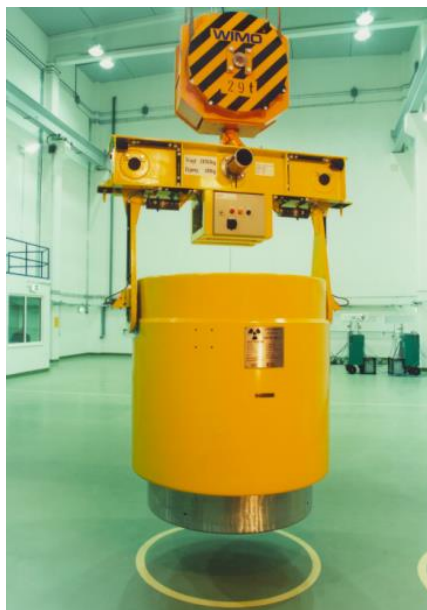
Figure 11: CASTOR ® MTR 2 for research reactor fuel
