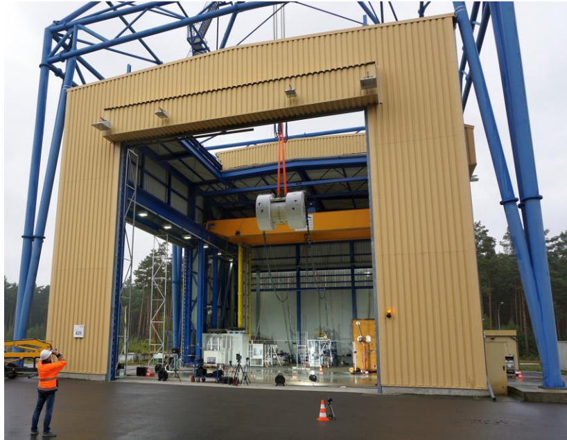
FIGURE 4. Drop test facility with test specimen ready for 9m-drop test.
