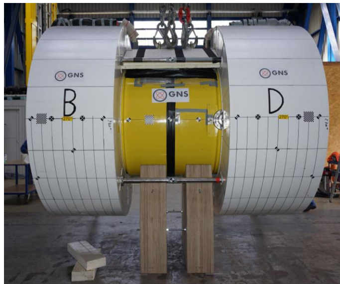
FIGURE 3. CASTOR ® MTR3 by Gesellschaft für Nuklear-Service mbH (GNS), Germany, and relating test specimen in horizontal drop test configuration.
