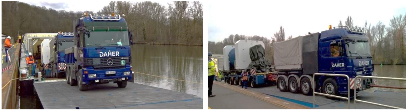
Fig. 12. Unloading Road Trailer with cask from river barge at the RORO berth of NPP Neckarwestheim.
