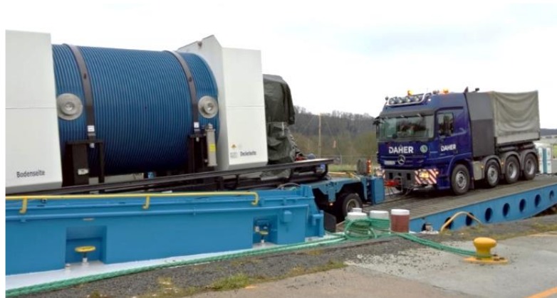
Fig. 8. Loading of cask type CASTOR® 440/84 mvK at the berth of NPP Obrigheim.
