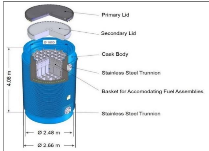
Fig. 1 Drawing of CASTOR® 440/84 mvK including dimensions.
