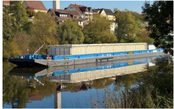
Fig. 7. River barge type LD40 after modification (incl. new security cover with blinds).
