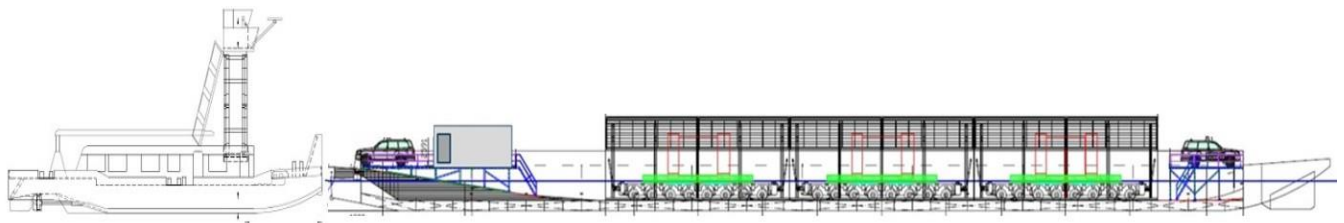
Fig. 4. Pusher tug and specially modified river barge type LD40 – also referred to as ‘pushing unit’.
