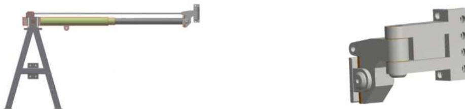
Figure 9 CAD concepts for the door closure system: [L] Hydraulic actuation and supporting frame [R] Additional hydraulic door clamping mechanism
