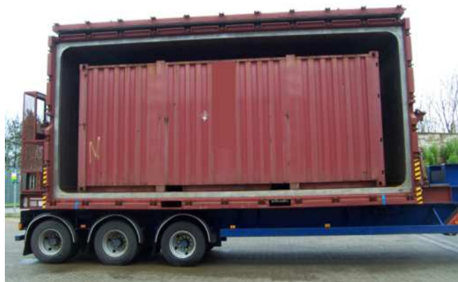
Figure 1 Existing oversized ISO container Type IP-2 transport package with the door open and ICC
