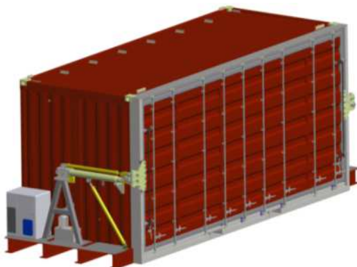
Figure 4 Concept oversized IP-2 container design CAD model showing the door and proposed hydraulic actuators
