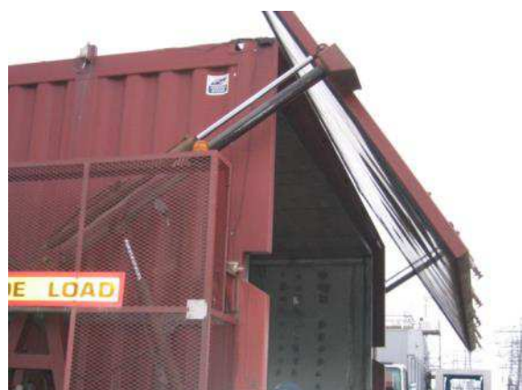
Figure 2 Door operations using Hydraulic Arms
