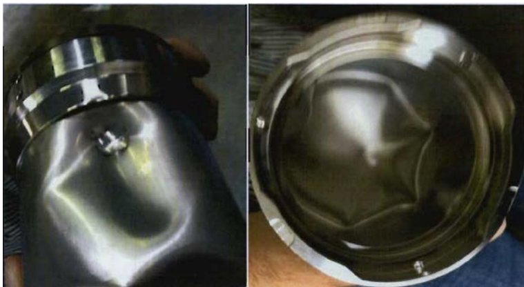
Figure 6. Damage caused by penetration bar test.
