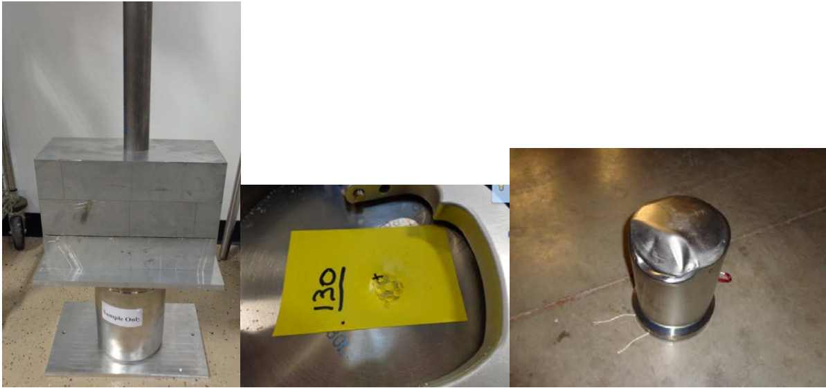
Figure 9. Results of the stacking, penetration and 30 Ft. drop tests
