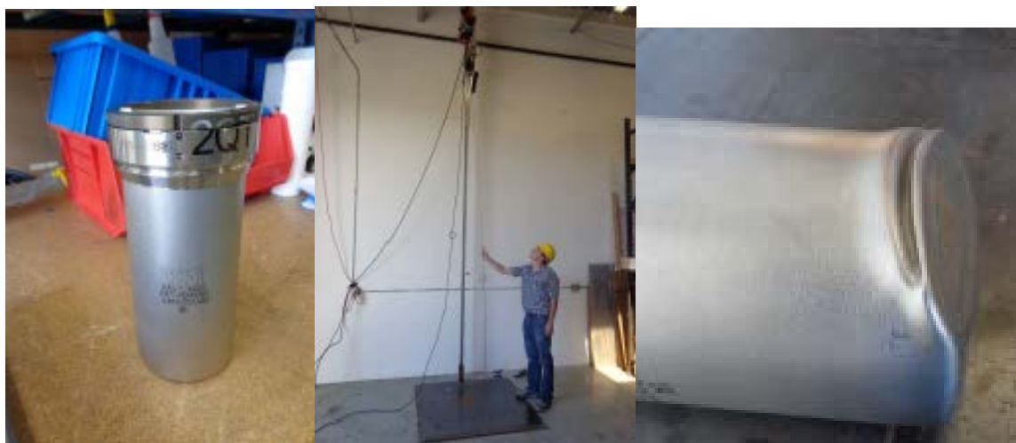
Figure 5. New 2 Qt. 12 ft. drop test and result.
