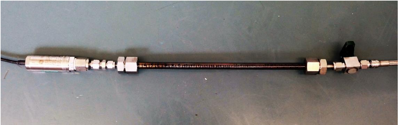
Figure 2 Pressurised hydrogenated Zr4 cladding tube used for the 3-point bending experiments.
