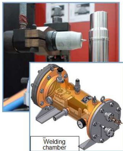
Figure 8 Qualified welding method and equipment for dry and welded capsule for DFR
