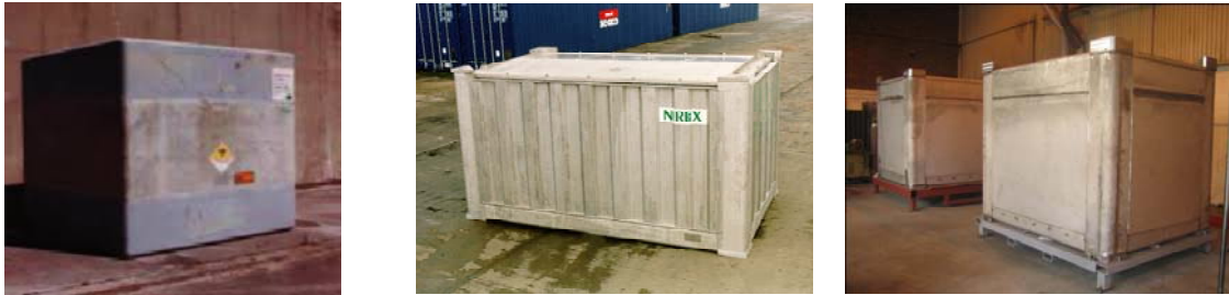
Figure 2. Shielded Waste Packages (6 cubic metre concrete box, 4m ILW box and 2m ILW box)
