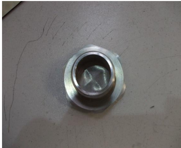
Figure 9 – Filter deformation post 20 bar burst test
