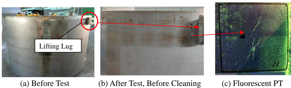
Figure 11 Results of VT and Fluorescent PT in area near the Lifting Lug
