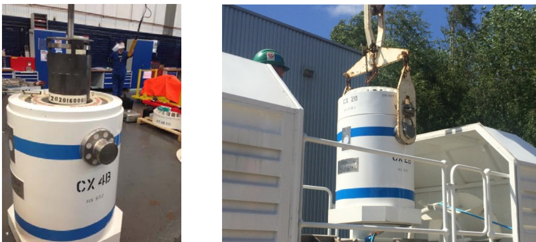
Figure 2 The loaded 28L disposable liner being lowered into the 1648C and then loaded to the transport trailer (Type A consignment).
