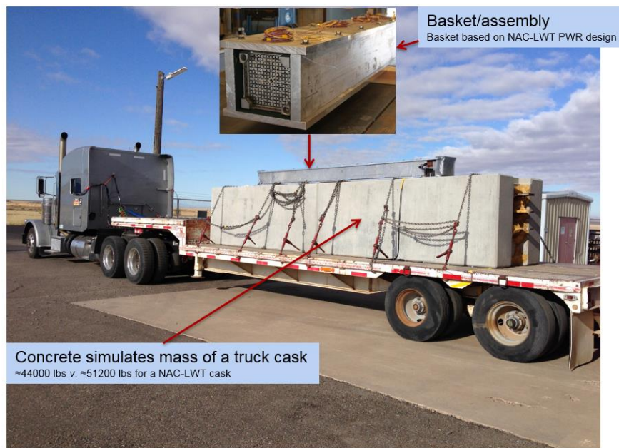
Figure 3 Over-the-road truck test configuration
