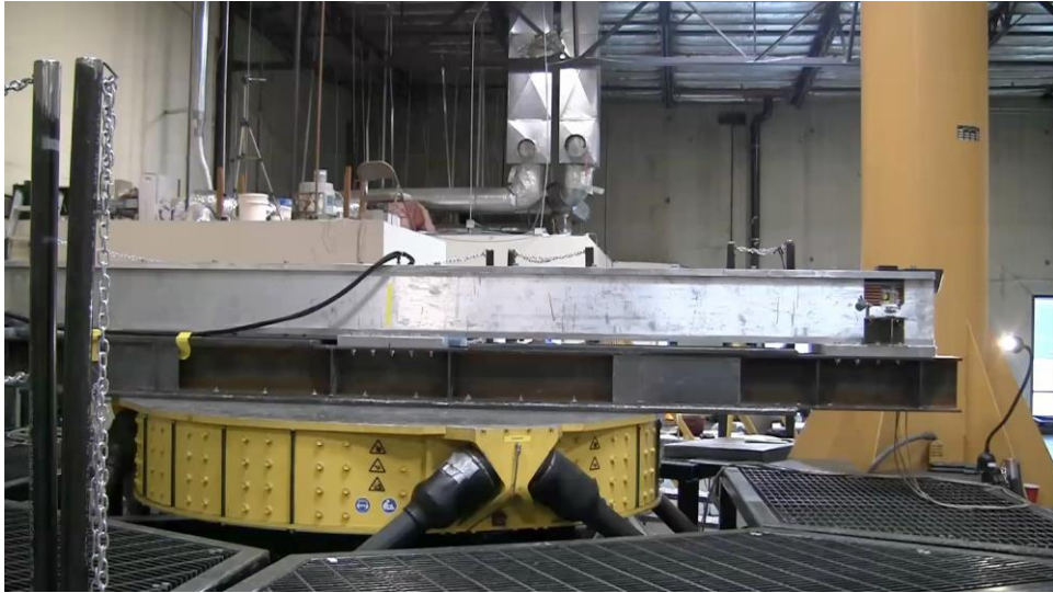
Figure 7 Multi-axis shaker used for rail and truck NCT tests
