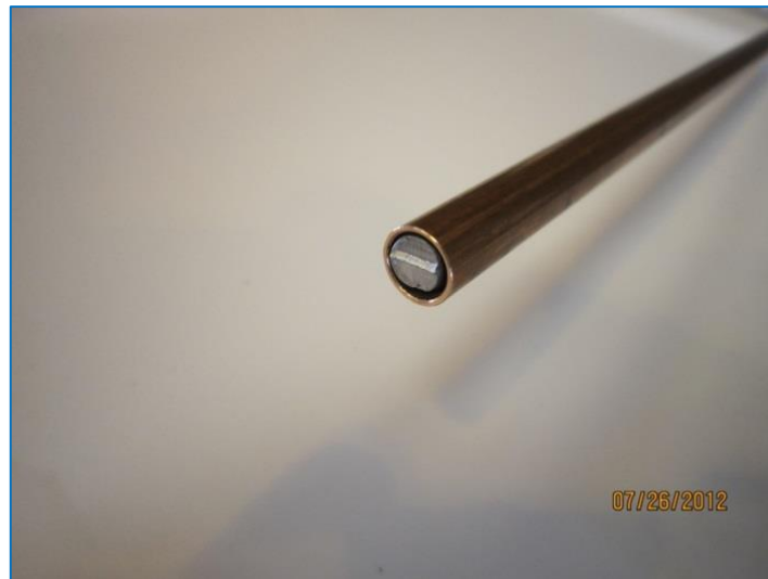
Figure 5 Lead “rope” with in copper surrogate fuel tube
