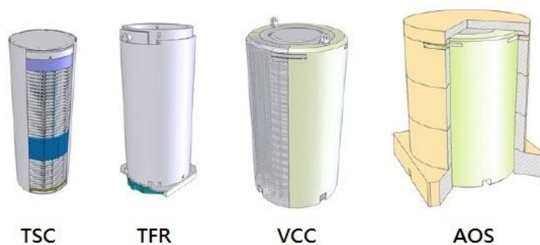
Figure 2 The major components of INER-HPS storage system
