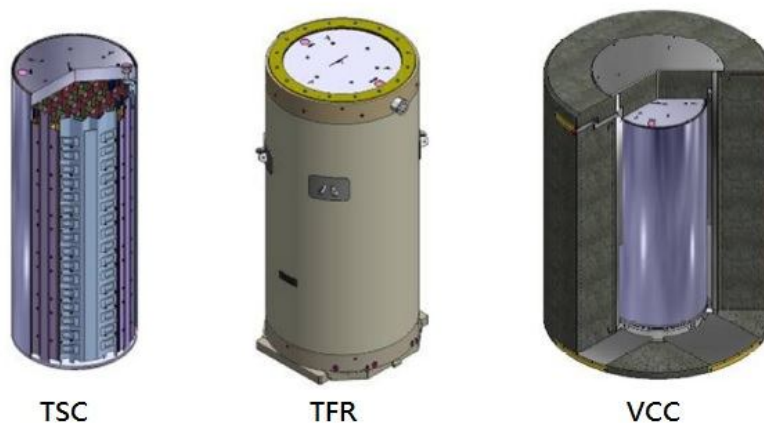
Figure 3 The major components of MAGNASTOR storage system
