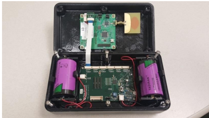
Figure 2. ACTS test units incorporate the DecaWave EVK 1000 Ultra-wideband module to perform IEEE 802.15.4-2011 communications.
