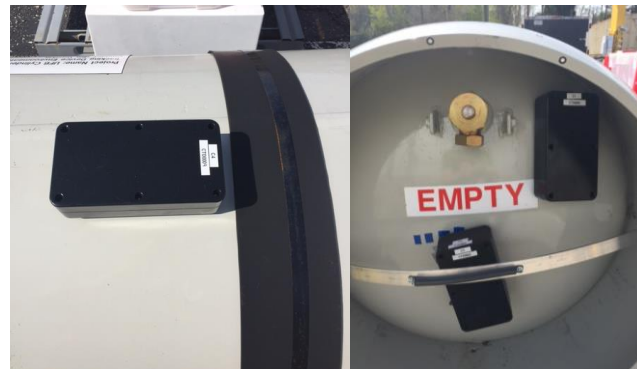
Figure 8. Outdoor 30B container device placement
