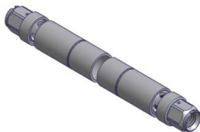
Figure 9 Tight capsule for defective fuel rod
