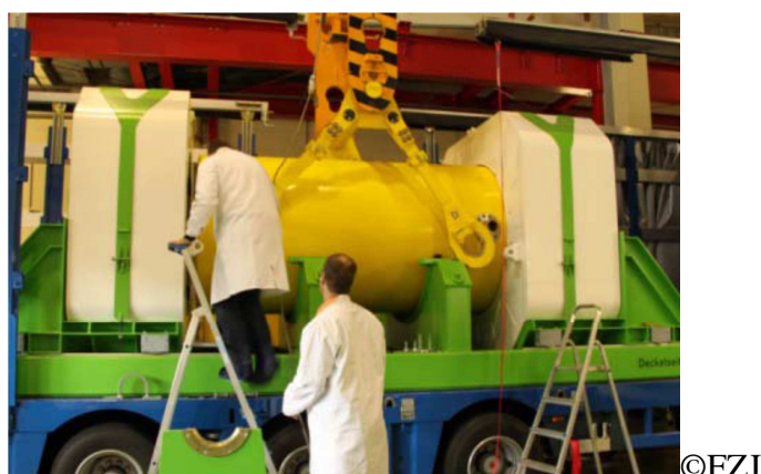
Fig. 6: Cask with Impact limiters on Transport Frame
