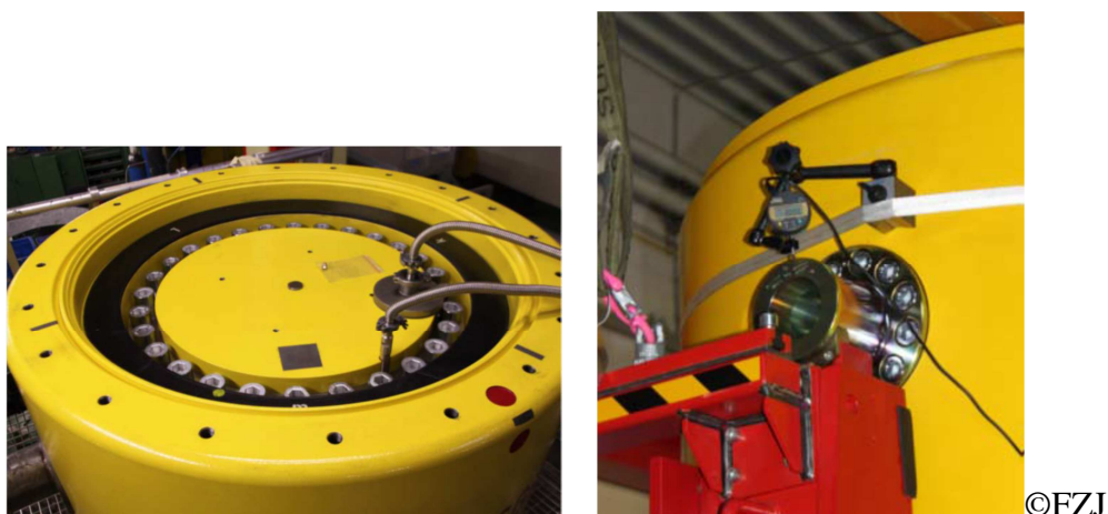
Fig. 7: Leak-tightness Test and Testing of Trunnions
