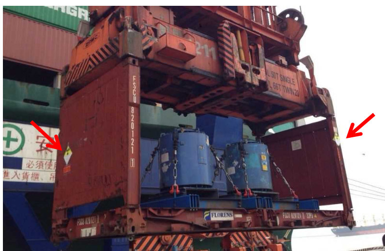
Fig. 4 Example of Placards affixed to an Open-type Freight Container
