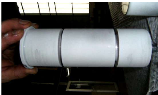
Figure 9 – Penetrant test on fuse pin
