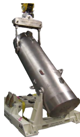
Figure 8 - IR200 cask and frame with tilting device
