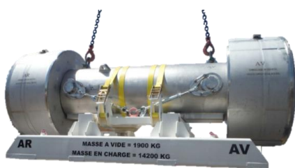
Figure 6 - IR200 cask with the new frame
