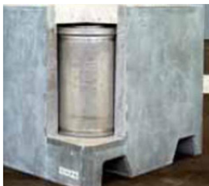
Dummy ILW-LL primary package in a section of its disposal overpack
