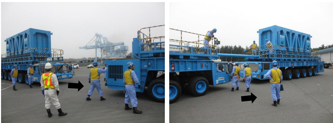
Figure 6. Carrier towing and pushing
