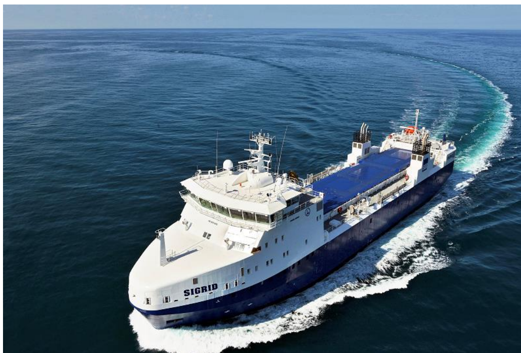
Figure 2 The INF-3 ship m/s Sigrid was taken in operation in the Swedish transport system in 2014. Photo: Damen. Source: SKB.
