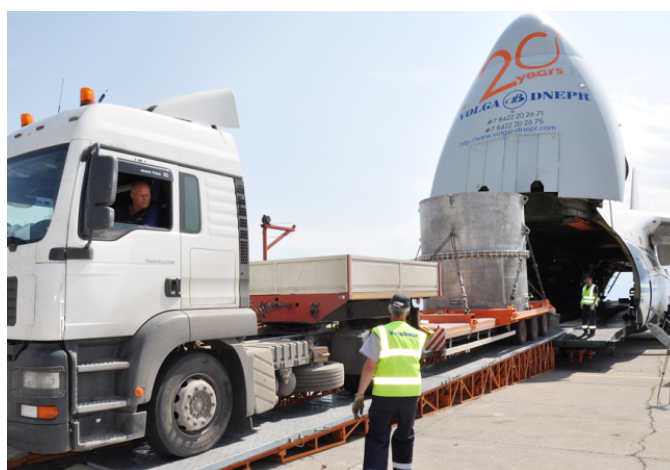
Figure 6 Special truck with TUK-145/C boarding the An-124-100 aircraft
