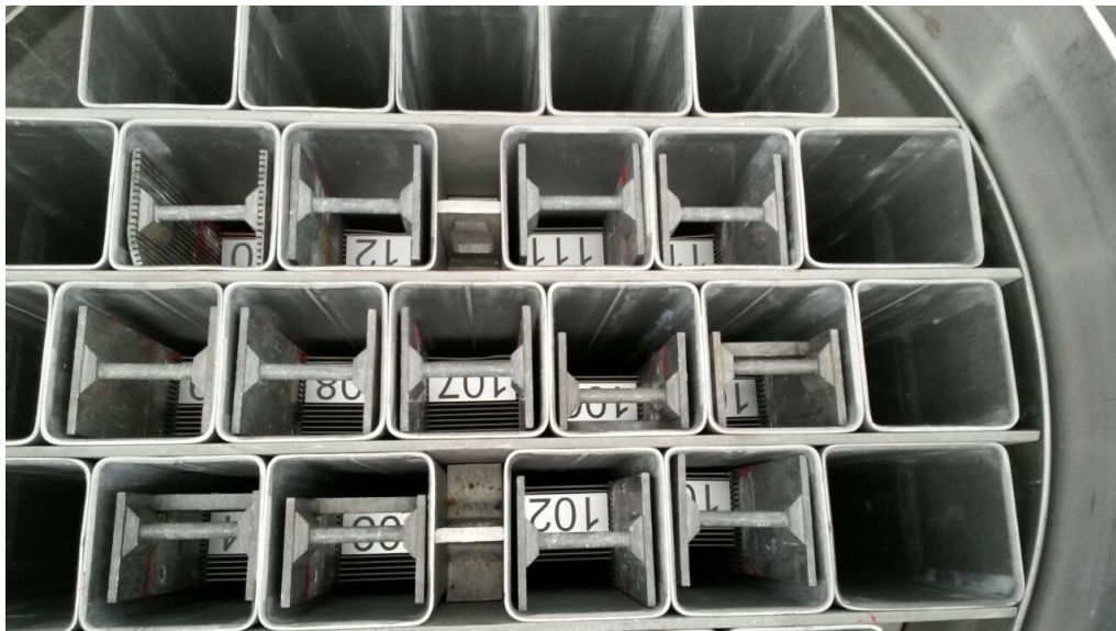
Figure 1: View of the basket of the packaging GNS16 loaded with fuel elements
