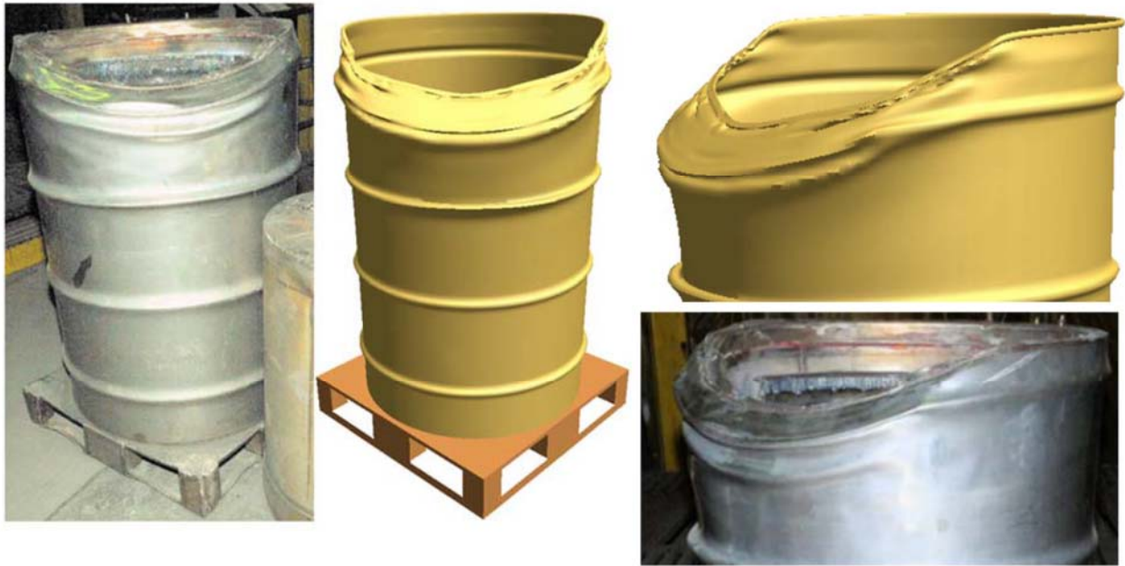
Figure 7 Lid edge drop – Drop test result vs analysis result
