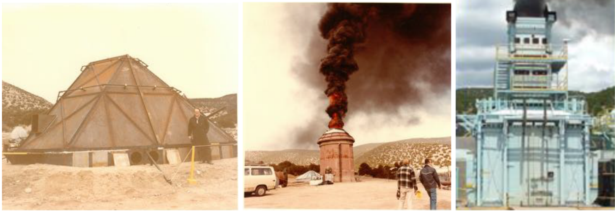
Figure 2. Left, the SWISH, a water-cooled wall enclosed pool fire facility for a 1 x 1 m pool. Center, the LAARC insulated wall enclosure for a 3 m dia pool fire with passive air control. Right, the SMERF, a water-cooled wall enclosure for a 3m x 3m pool with active air control.
