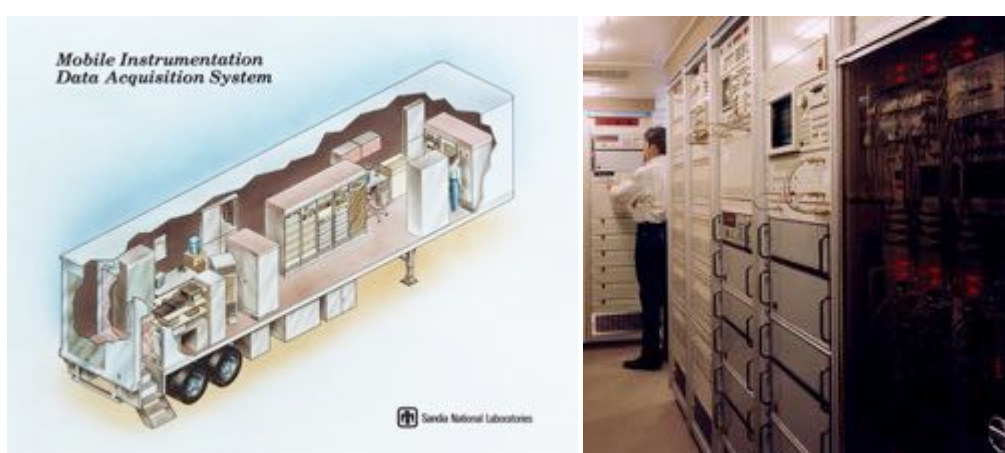
Figure 9. The MIDAS is fully mobile and supports package testing at worldwide sites. This unique self-contained mobile system is capable of acquiring and processing up to 168 channels of piezoresistive or voltage based transient structural data. In addition, up to 100 channels of temperature data can be collected and processed.
