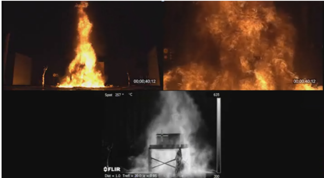
Figure 4. A set of 30-gallon shipping drums in a 3 m diameter fire in the FLAME facility. The visible and IR views clearly demonstrate full engulfment of the test items.
