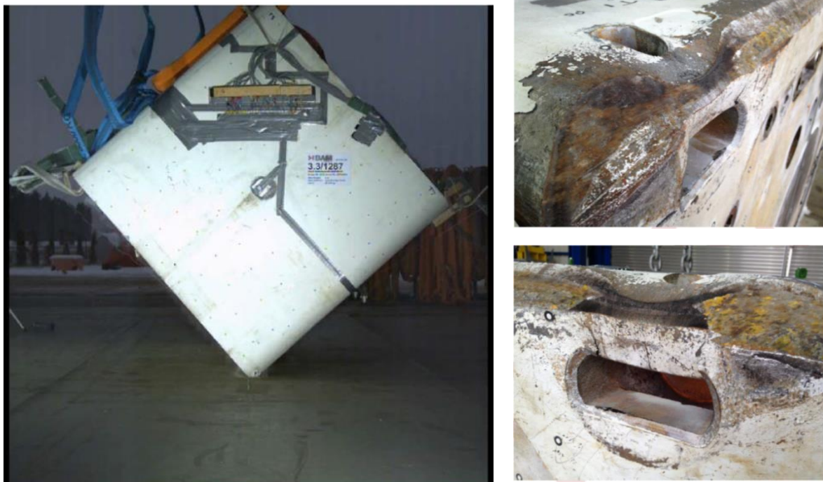
Figure 5 – Pictures from full-scale drop test of Safstore DCI container
