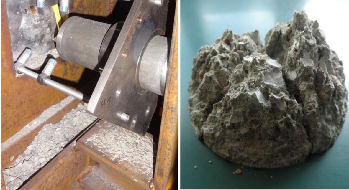
Figure 7 Photographs of the disintegrated cement cylinder target. (Test #2, 50 g explosive)
