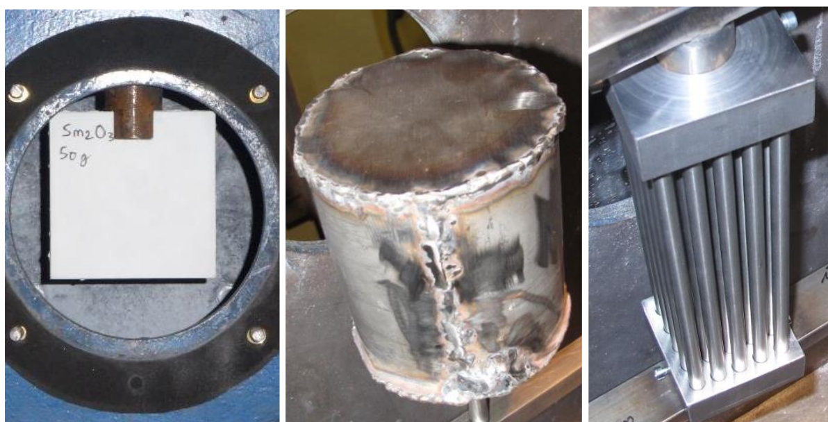
Figure 5 The three different target configurations used in the tests: ceramic plates
