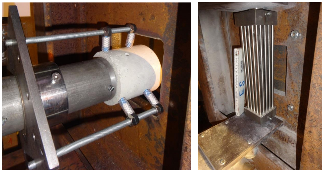
Figure 2 Cement cylinder target setup “inside” (left) and fuel mock-up “inside” (right)
