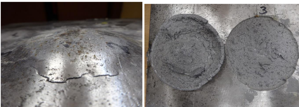
Figure 8 Photographs of the damaged stainless-steel plate after interaction with the small explosive charge. Left: deformation for a distance of 1 mm between plate and target. Right: deformation for a distance of 33 mm between plate and target.
