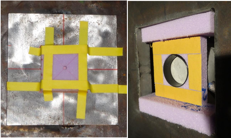
Figure 3 Stainless-steel plate with mounted explosives “outside” (left) that were used as a mock-up of a transport cask and mounting for explosives which is put on the target (right)
