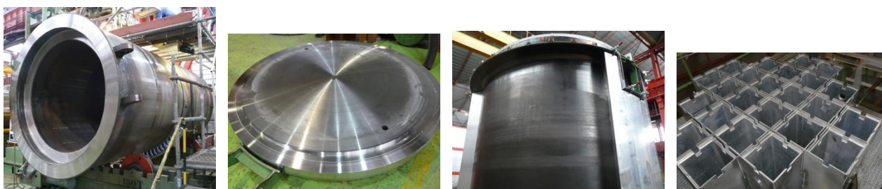
Figure 7 Final Design and Manufacturing Sequences of the ENUN 24P
