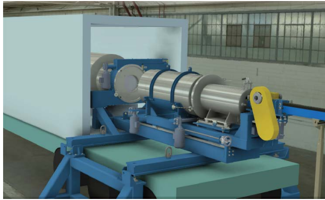
Figure 4 UNL Canister Horizontal Loading
