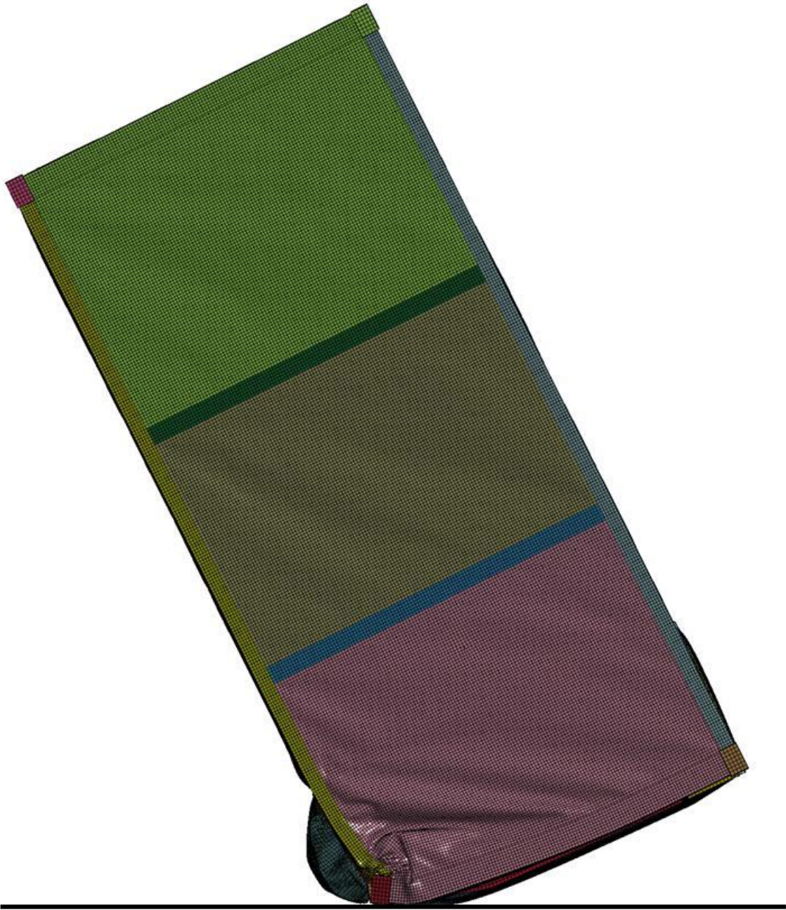
Figure 4 Deformations of the calculation model after the 9 m drop on the front edge
