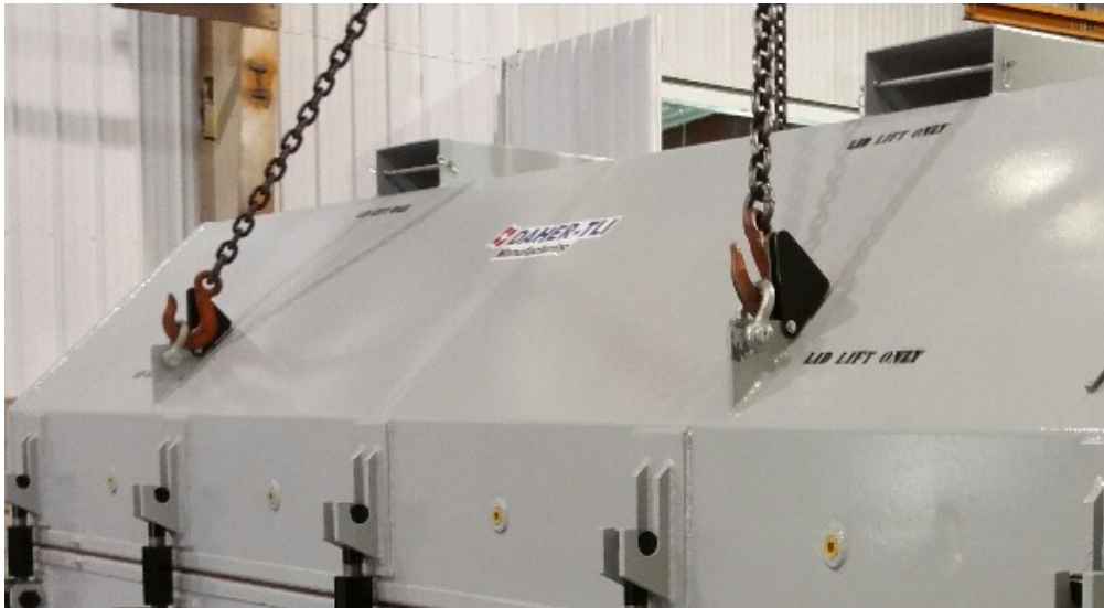
Figure 6 – Lifting the Kevil Kougar Upper Subassembly with Lifting Lugs
