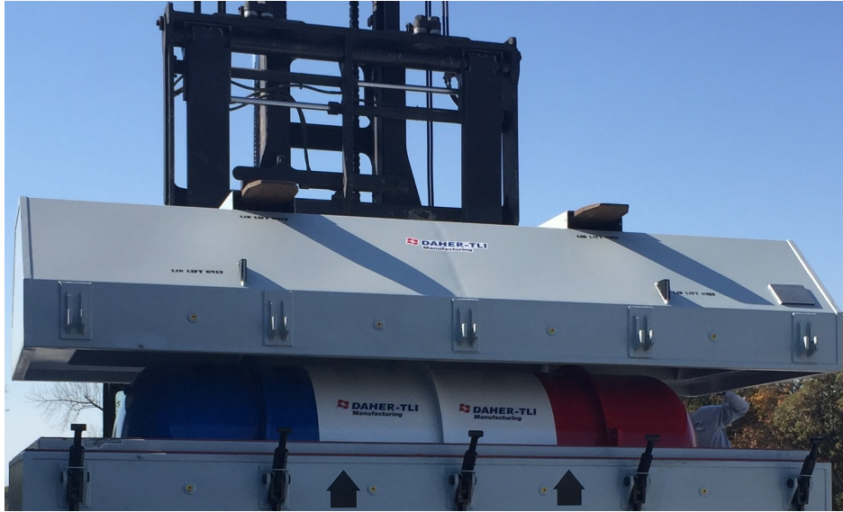
Figure 5 – Lifting the Kevil Kougar Upper Subassembly with Fork Lift Pockets
