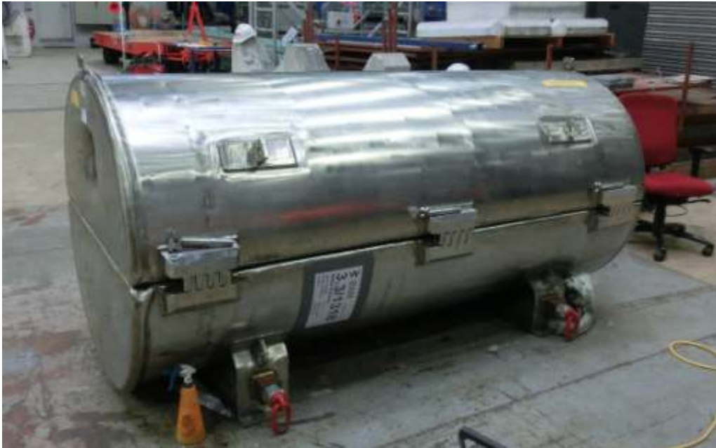
Figure 5: DN30 prototype after drop test sequence 3
