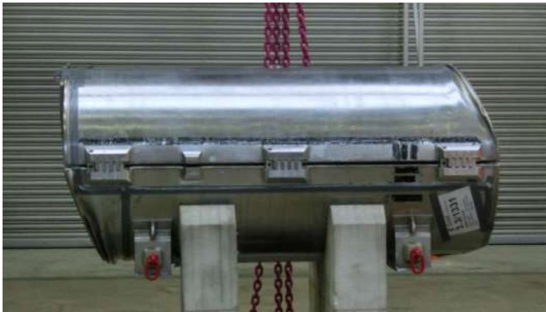
Figure 4: DN30 prototype after drop test sequence 1 followed by drop test sequence 2
