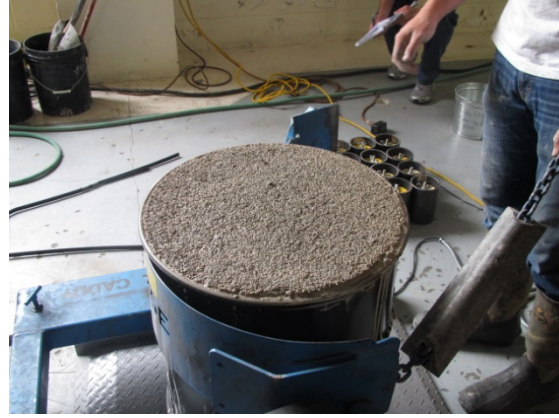
Figure 4. Simulated MD-2 drum casting sample (before and after casting).
