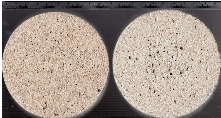
Figure 2. Discs of Kaolite (on left) and Packcrete after baking.
