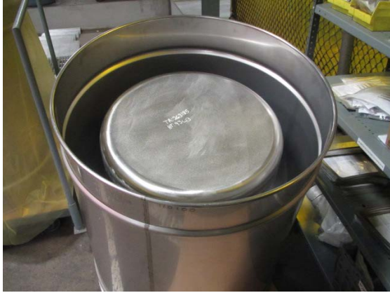
Figure 4. Simulated MD-2 drum casting sample (before and after casting).
